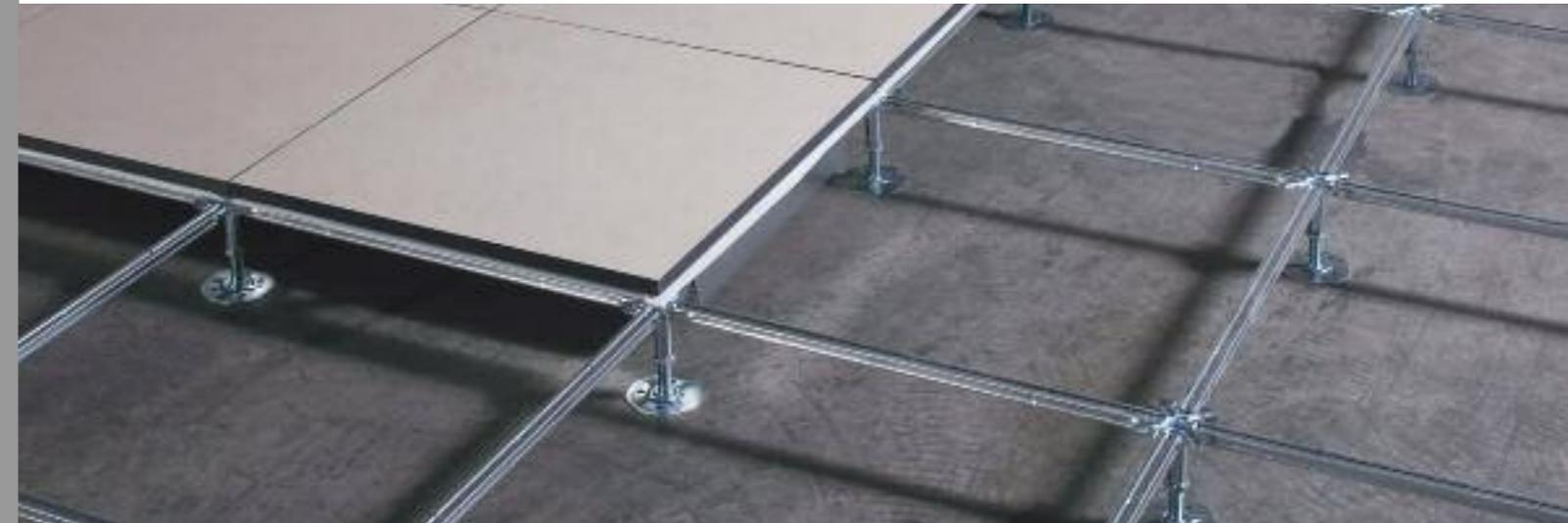
*PETRAL supplies galvanized steel pedestals. The head of the pedestal is predisposed for the wedging of the stringers, and is equipped with a gasket, as are the stringers. The height of these structures is adjustable from a minimum of 3,5 cm to over 100 cm. We offer five types of structures according to different load requirements: SA - ST1 - ST2 - ST3 - ST4.*
