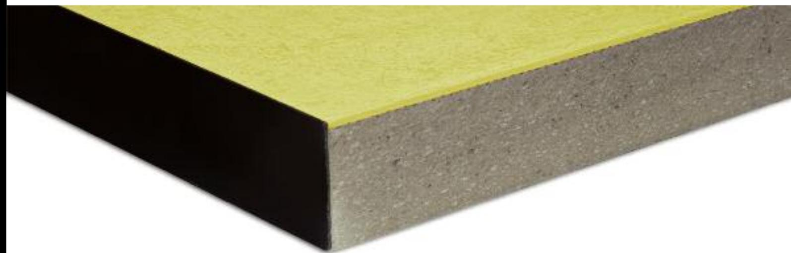
*High density, single layer, modular panel made of chalk and cellulose fibres. In its standard thickness of 30 mm, it is ideal for a Porcelain Tile finish while the 34 mm is suitable for a HPL and resilient finish. It presents elevated physical and mechanical performance, high resistance to fire and sound and it can be accompanied by any type of finish.*
